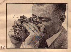
For pictures in the half-size,  $2\frac{1}{4} \times 1^{5}/s$  in., bring up the small side mask into the frame; this mask is hinged to the front portion of the finder.
